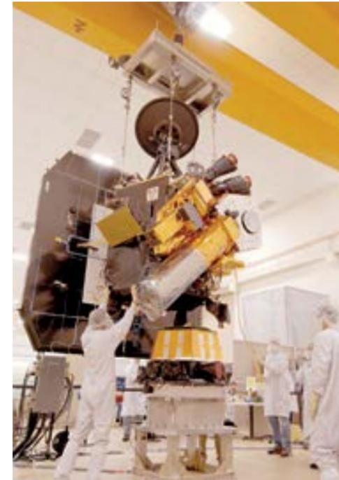
▲ Engineers at the Ball Aerospace plant in Boulder, Colorado, pictured here in the process of joining the Deep Impact flyby spacecraft to the impactor
